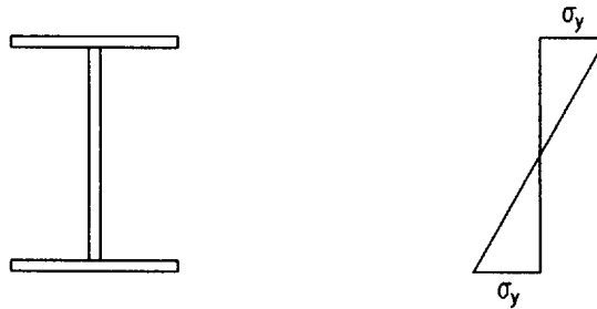
Fig. 17.11 Design stresses for non-compact sections
